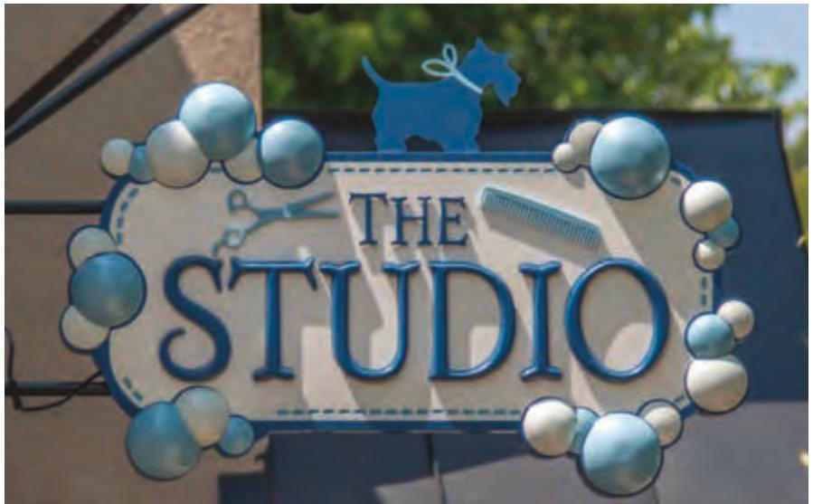
3-ft.-wide HDU sign with carved HDU soap bubbles. Integral aluminum structure has a custom bracket with down lights. Three LED fixtures are integrated into bottom to light walkway and entrance. Photo by Dragon Ridge Photography
