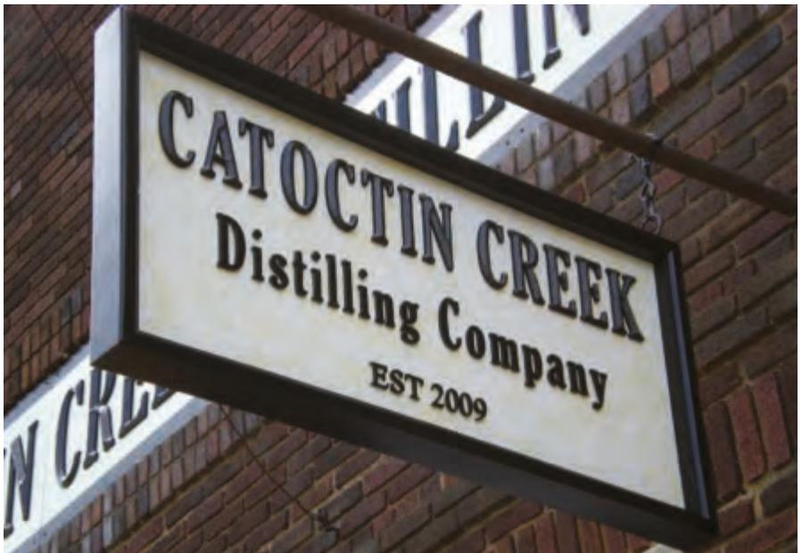
4-ft.-wide aluminum composite panel with faux antique finish; router-cut HDU letters were hammered with a ballpeen hammer before finishing with Matthews Paints [www.matthewspaint.com].
