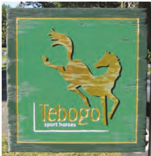
3-ft. carved HDU sign. The raised acrylic horse was cut on the Epilog laser cutter, and the panel was aggressively distressed with wire wheels and brushes.
