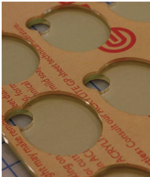
Besides engraving, lasers are impressive cutting tools, which is handy for sign work. It leaves acrylic with a smooth, finished edge as you can see here.
