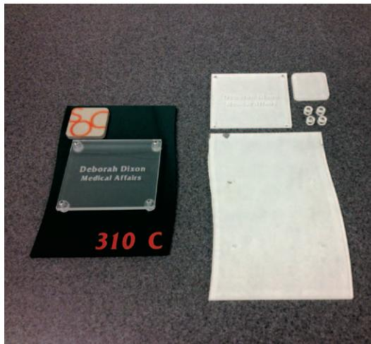
You can see that we cut all the components for this rather complex door sign on the laser from a single piece of acrylic—even the standoffs.
