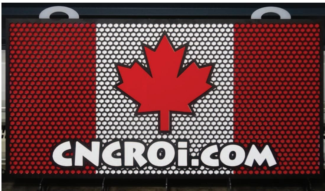
**Jon Cantin, CNCROI.com, fabricated** this 15-by-30-in. trade show display using his Trotec laser. The black 1/8-in. acrylic layer is mounted to the red and white 1/8-in. acrylic, which is backed up with 1/4-in. acrylic. You can watch a video of how he produced it by visiting Jon's blog at [www.cncroi.com](http://www.cncroi.com) and scrolling down to "New Acrylic Signage for CNCROI.com". Based in Canada, Jon provides custom CNC laser and router services.
